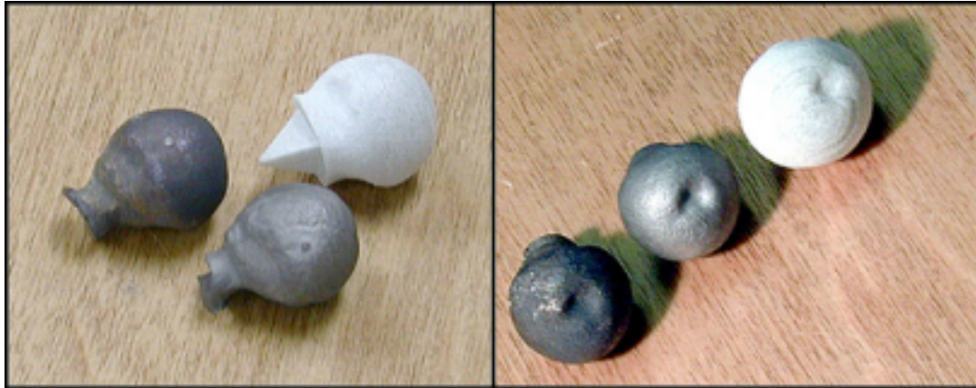
Above pictures of 2 titanium cast (dark) and 1 nylon (white) ball with insert.
